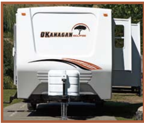
ECL29RBS showing one-piece moulded fibreglass cap
